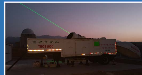
The mobile SLR system (TROS) in Xinjiang Observatory (Urumqi)
